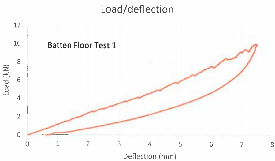
Figure 2. Load/deflection plot, test 1
